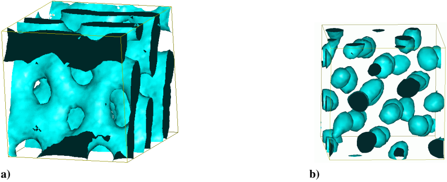
Fig. 8. a) Perforated lamellar system for \langle f \rangle = 0.35 , after [36]. b) Body-centred cubic system at \langle f \rangle = 0.14 , after [36]
